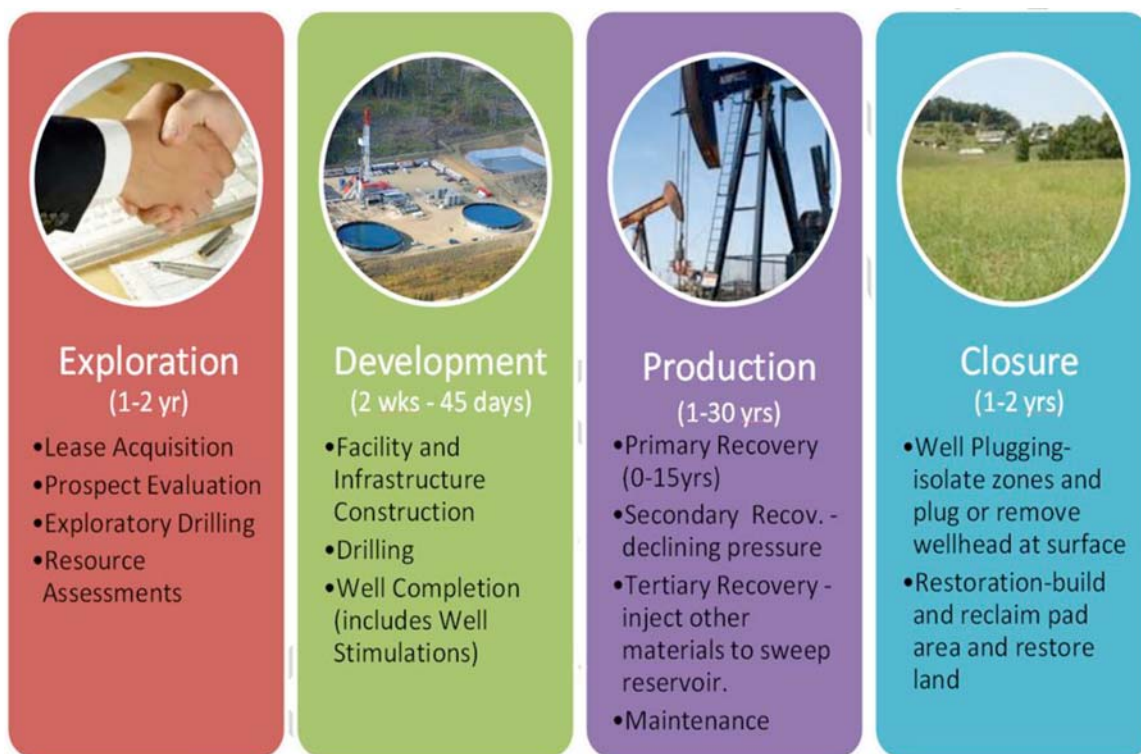
FIG. 1 Phases of Oil and Gas Development Operations Well Life Cycle
